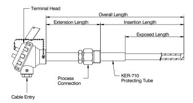
PROTECTION TUBE THERMOCOUPLE ASSEMBLY
